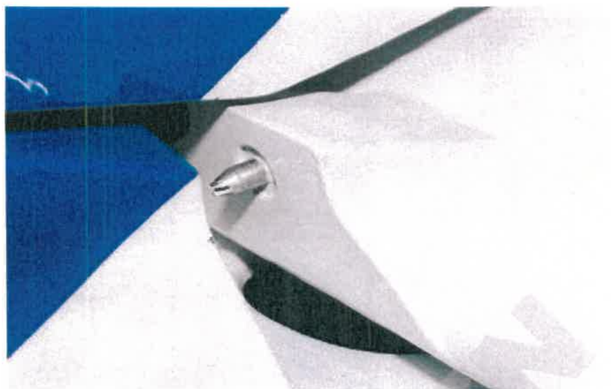
View 8-7 Entering the horizontal stabilizer dowel to fuselage seat
